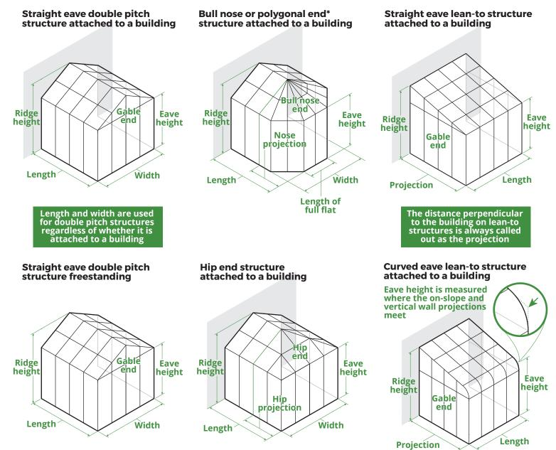
Note: when there is no transom, the eave height is determined by the thickness of the frame. \* Also referred to as a conservatory nose
