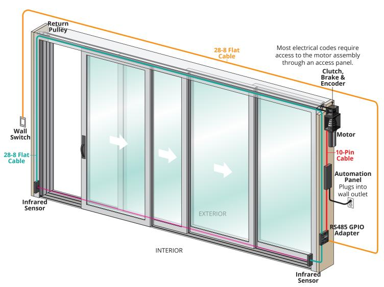
The Automation Panel and Adapter must be installed within six feet of the Motor.
